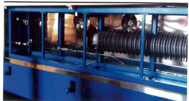
BENDING MOMENT TEST ON 156kV TUBE DESIGN S.A.
