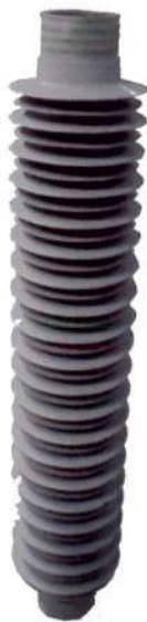
Hollow core Insulator after moulding
