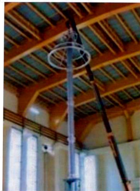
SEISMIC TEST ON 624kV 20kA class-V POLYMER SURGE ARRESTERS
