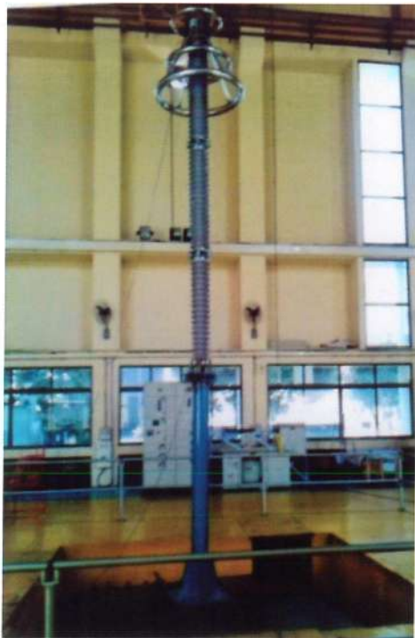
SEISMIC TEST ON 360kV CAGE ARRESTERS
