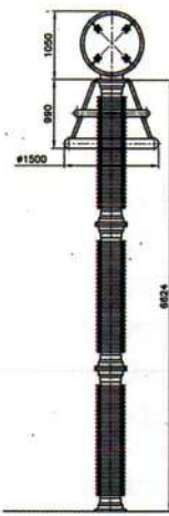
624kV SA(3 UNITS)
