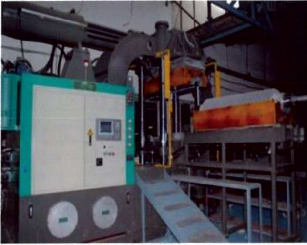
EJECTION OF PRODUCT AFTER INJECTION MOULDING INJECTION MOULDING OF HOLLOW CORE INSULATOR AND CAGE DESIGN OF ARRESTER
