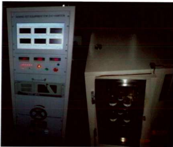
LONG TERM STABILITY TEST (Accelerated ageing test) at 115^{\circ}\text{C} AC or DC upto 6kV
